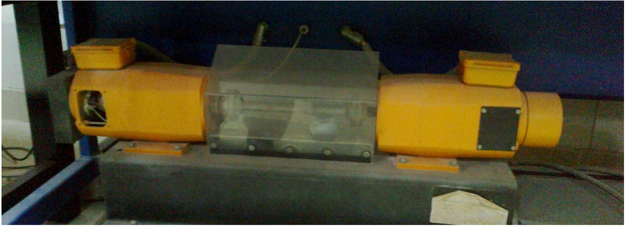
Fig: Motor and Alternator of Scan Drive System
